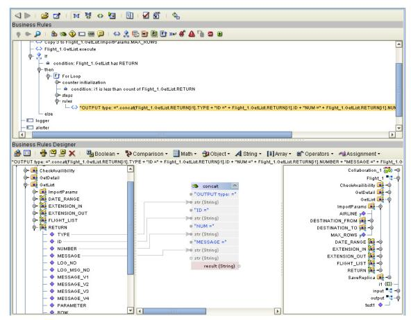
7 Connect the result (String) in the concat to the test1 field, located under jcdFlightGetList > output.
